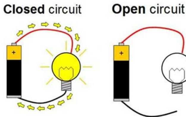
This same concept is used when using an on/off switch for a circuit. The “on” position produces a closed circuit and the “off” position provides an open circuit. The on/off switch is often symbolized with an icon (see icon image below). Similarly, the (a) diagram is switched on and the (b) diagram is switched off.
